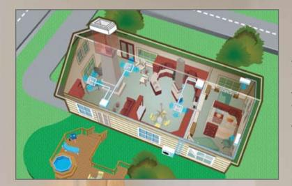
Daikin's new generation 2-port, 3-port and 4-port Multi-Split Systems are able to serve 2, 3 or 4 zones (rooms) from over 200 possible combinations. Choices include: all wall mount units, all slim duct units or a combination of both. With energy efficiency up to SEER 19.5 and HSPF 9.5, these systems will enhance the comfort of any home and also be easier on the electric bills.
