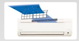
Activated by the exposure to natural light, the titanium apatite photocatalytic air purification filter traps microscopic particles, decomposes odors and absorbs and deactivates bacteria. This filter lasts for three years with proper maintenance.
