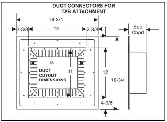
FIGURE 4: Duct Connector Dimensions (7990 Series)
