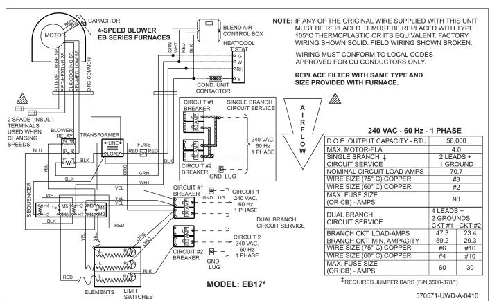
FIGURE 19: EB17\* Wiring Diagram
