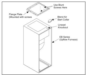
FIGURE 11: Blower Bracket and Duct Flange Attachment WIRING
