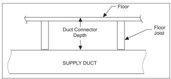
FIGURE 3: Duct Connector Depth (7990 Series)
