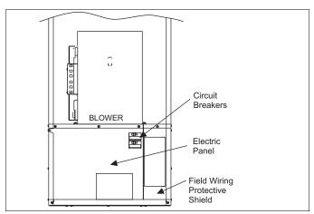
FIGURE 13: Field Wiring Shield
