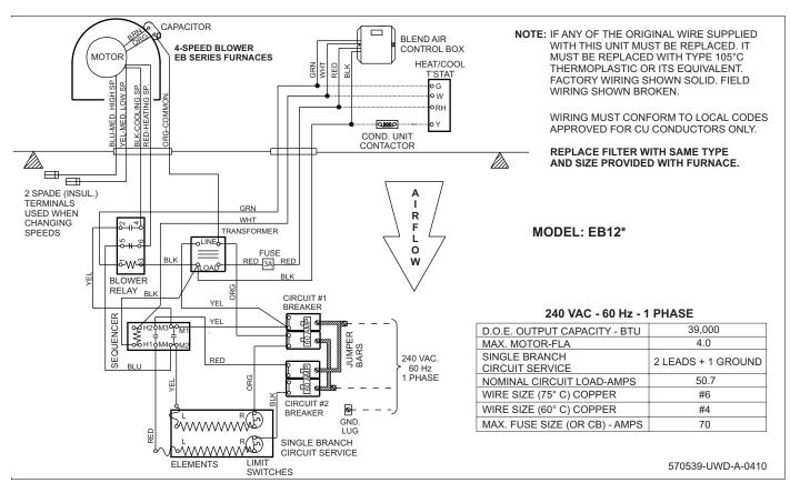
FIGURE 17: EB12\* Wiring Diagram
