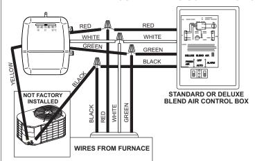
Four-conductor wire is required for thermostat connection. Attach the 4 low voltage wires extending from the control box as follows:
