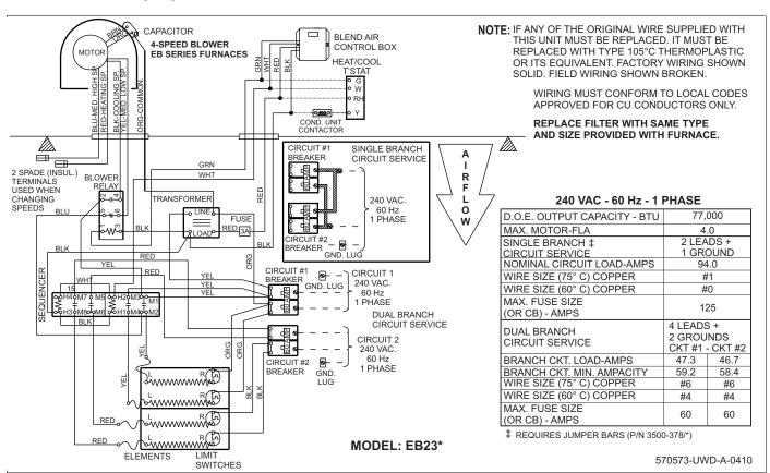
FIGURE 21: EB23\* Wiring Diagram
