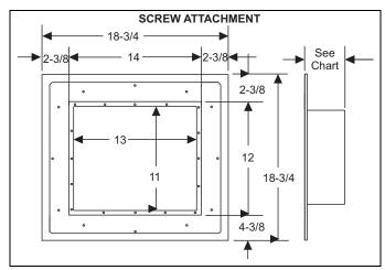
FIGURE 4: Duct Connector Dimensions (7990 Series)
