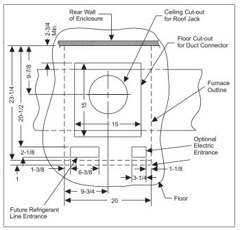
FIGURE 5: Recommended Floor Cut-out (7990 Series)
