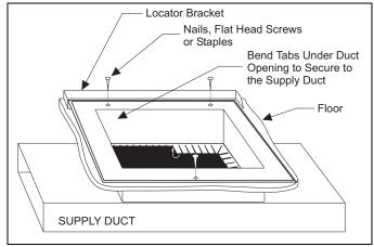
FIGURE 7: Duct Connector Tab Attachment (7990 Series)
