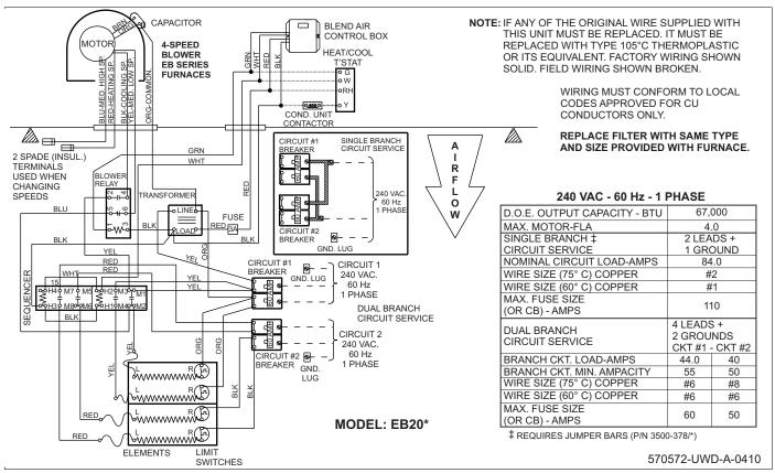
FIGURE 20: EB20\* Wiring Diagram
