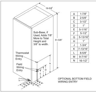
FIGURE 1: Furnace Dimensions
