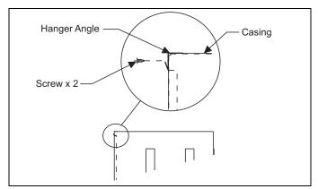
FIGURE 10: Hanger Angle Attachment
