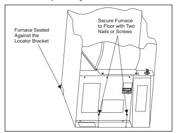
FIGURE 9: Installation of Furnace
