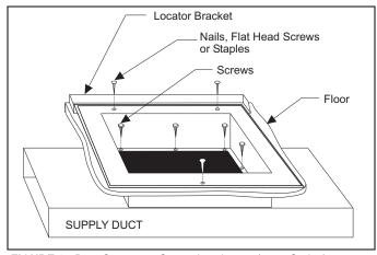
FIGURE 6: Duct Connector Screw Attachment (7990 Series)
